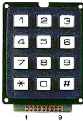
Pins 1 and 9 are unconnected - only pins 2 - 8 are used.
